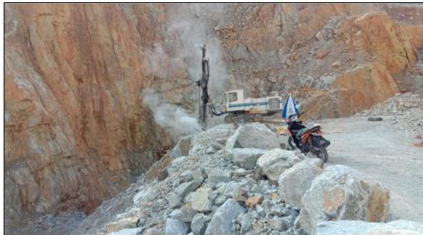
Rock Drilling & Blasting Work
