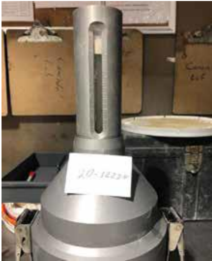
Fig. 7: The microsphere content of a concrete mixture can be evaluated using a volumetric meter
