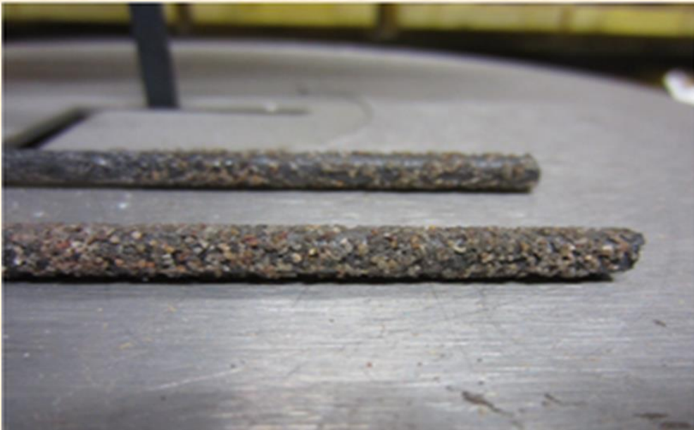
Image 1: Photograph of sand-coated CFRP tendons (Source: Dr. Shobana Sivanendran)
