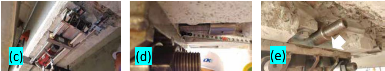
Fig. 6: Post-tensioning of NSM CFRP: (a) mounting of hydraulic ram in the jacking apparatus; (b) inserting a load cell between the ram and bracket; (c) completed jacking apparatus during operation; (d) measurement of elongation at jacking-end; and (e) fastening nut adjusted to lock-in post-tensioning force prior to removal of jacking apparatus.
