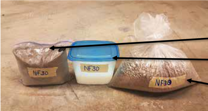
Fig. 3: Prepackaged constituents for NMFC mixture NF30 Binder(cement and fly ash) Liquid phase (water, nanosilica, and admixtures) Aggregates(natural gravel and sand)
