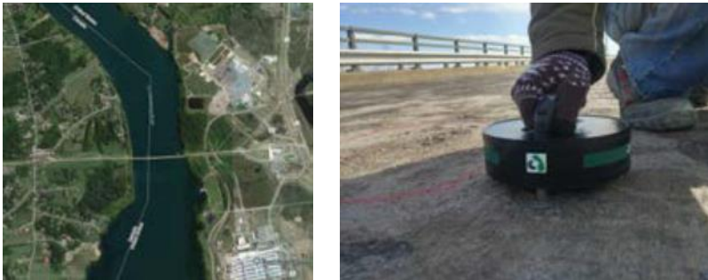
Fig. 1: The Three Nations Bridge was evaluated using visual, acoustic, and electrochemical measurements: (a) aerial view of Cornwall Island, ON, Canada (left) and Akwesasne, NY (right); and (b) closeup of the device used to take electrochemical measurements
