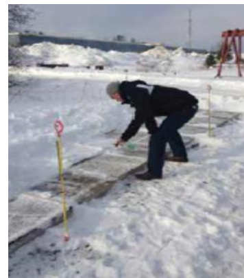
Fig. 2: Spraying slabs with NaCl solution at the UNB exposure site
