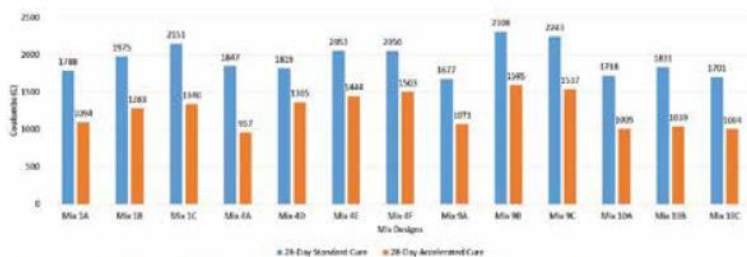
Fig. 2: ASTM C1202 RCPT results for PLC concretes containing Class F fly ash
