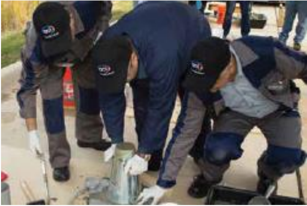
Slump test being performed by University of Technology–Baghdad professors
