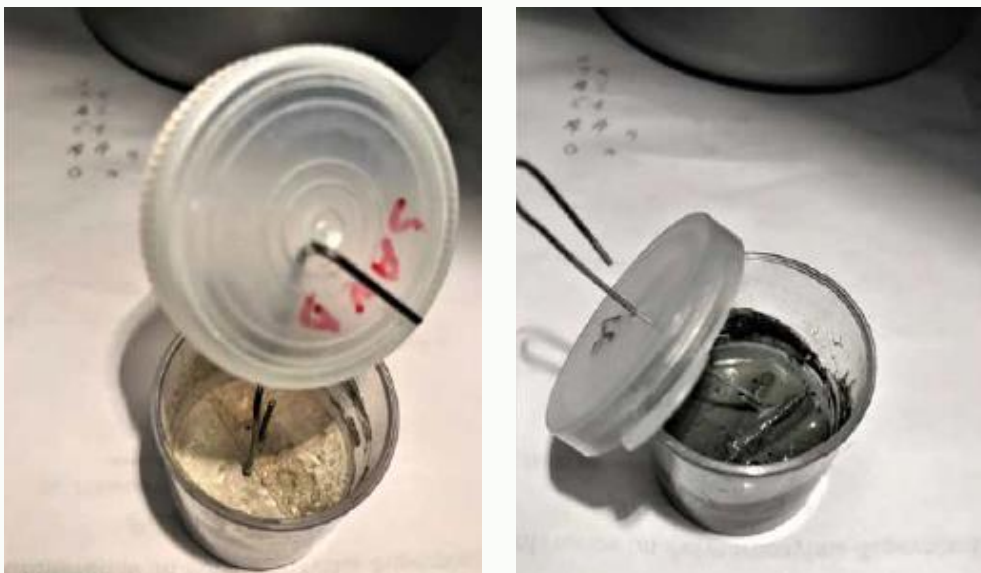
Fig. 3: Three-day-old mortar samples prepared with: (a) water; and (b) sucrose solution
