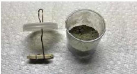
Fig. 2: A 25 mL vial with a cement and sand mixture. The vial cover was fitted with a paper clip affixed to a small clothespin
