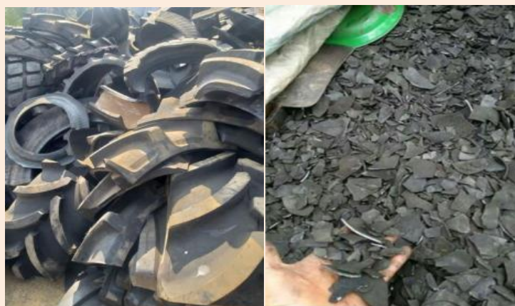
Figure 2: Waste tyres and tyre chips [5]
