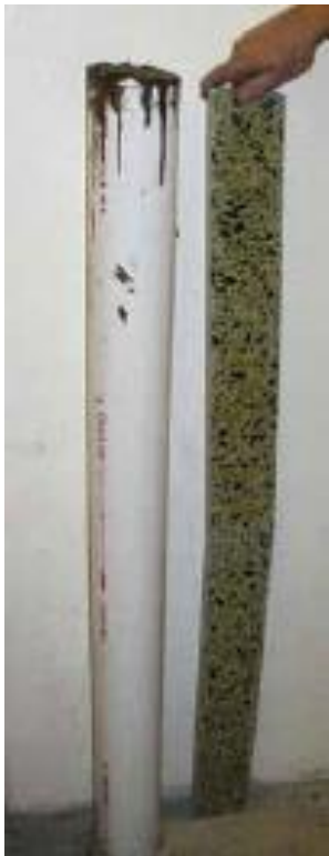
Fig. 3: The stability (resistance to segregation) of an SCC mixture was evaluated by casting a 4 ft (1.2 m) tall column in a PVC pipe, allowing the SCC to harden, and cutting the column in half using a masonry saw. A uniform distribution of coarse aggregate over the height of the column demonstrates that the mixture is stable
