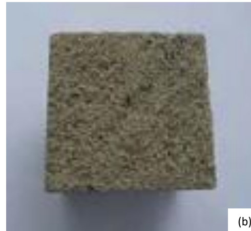
Fig. 7: Shotcrete samples—two-layer concrete with an external pale yellow architectural coat made according to the “cut” technique: (a) cross section; and (b) finished surface
