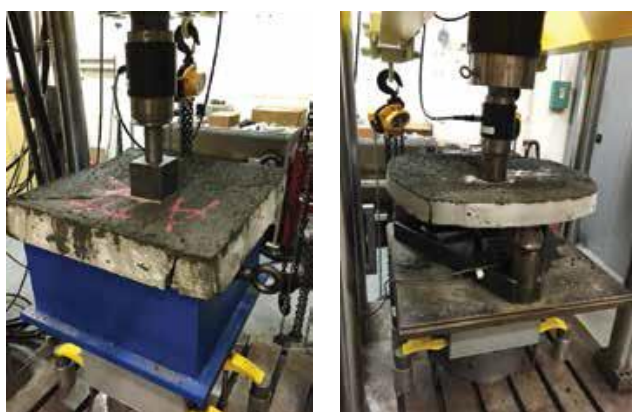
Fig. 1: Setup for bending tests: (a) ASTM C1550; and (b) EN 14488-5 11 test methods
