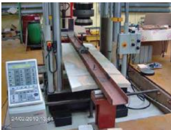
Fig. 5: Structural testing of a 2.10 x 0.80 x 0.05 m (83 x 32 x 2 in.) panel cut out from a mockup wall. Anchors were spaced at 0.8 m (32 in.) and load was distributed by the steel channel in the center
