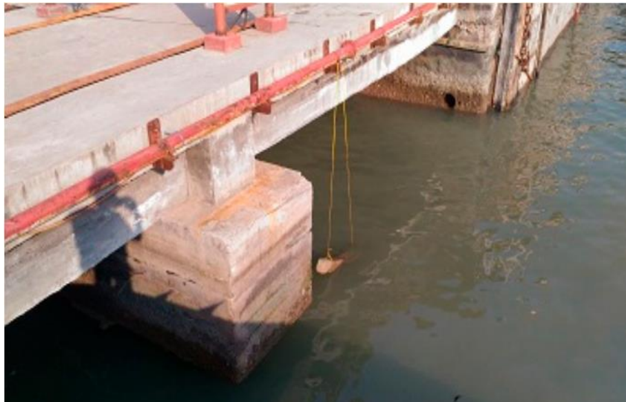
Figure 3: Geopolymer concrete beam cured in seawater for 28 days [32]
