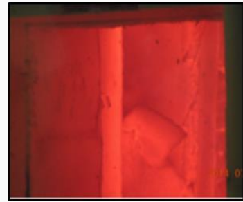
Fig. 7. Image of column during ASTM E119 fire test captured from the viewport of furnace
